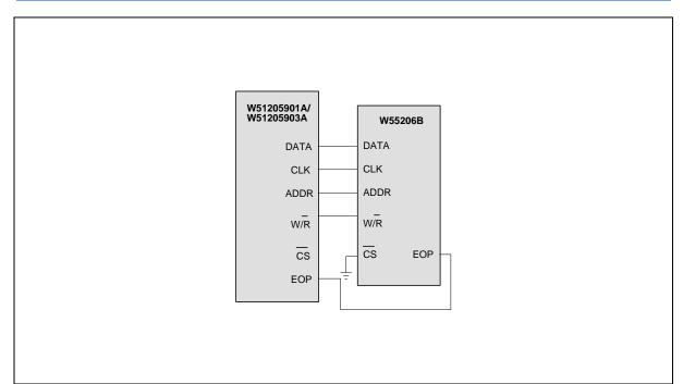
\* W51205901A/W51205903A substrate connected to Vss for C.O.B.
